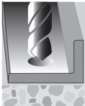
1. Mark and drill the drilling position ( \varnothing 12 mm)
