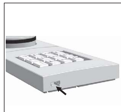
Figure 10: Mini-USB socket Special interface, only in connection with original Kaba Mauer CB30 Use PC cable!
